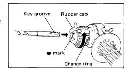
Turn the change ring in the direction of the arrow until the mark on the change ring is aligned with the mark on the rubber cap to secure the bit.
